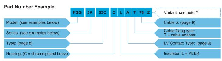
**FGG.3K.03C.CLAT76Z** = Straight plug with key (G), 3K series, multi-fibre type to accept 4 F7 type fibre optic contacts, chrome-plated brass housing, PEEK insulator, cable fixing type T for 7.5 mm diameter cable, and nut for fitting a bend relief.
