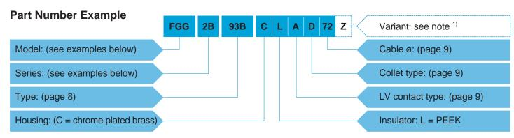
FGG.2B.93B.CLAD72Z = Straight plug with key (G), 2B series, mixed type to accept 2 F7 fibre optic contact and 4 low voltage electrical contacts, chrome-plated brass housing, PEEK insulator, 4 male solder electrical contacts, type D collet system to suit a 7.0 to 6.1 mm diameter cable, and a nut for fitting a bend relief.
