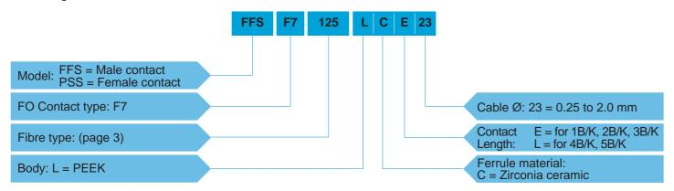
FFS.F7.125.LCE23 = Male F7 type fibre optic contact, ferrule bore diameter of 125  $\mu$ m, PEEK body, Zirconia ceramic ferrule, contact length for 1B/K, 2B/K or 3B/K series, for cable with diameter max = 2.0 mm.
