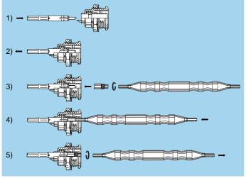
For female contacts, the alignment device shall be clipped onto the fibre optic contacts which is already fitted into female insulator. This procedure is performed using the tool, reference DCS.F7.035.PN. The alignment device shall be first installed onto threaded end of the tool (step 3). Then clip the adapter (step 4), unscrew and remove the tool (step 5).
