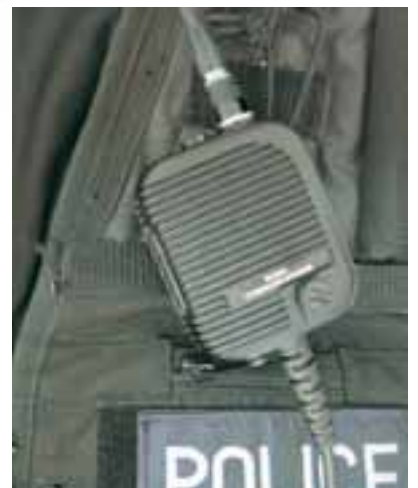
Firearms Remote Audio Terminal with K series connectors. (Sonic Communications Ltd, UK)
